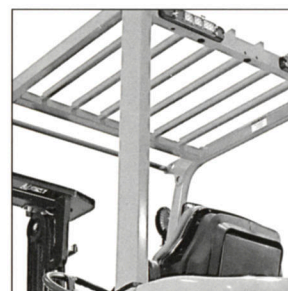
Clear-view overhead guard
